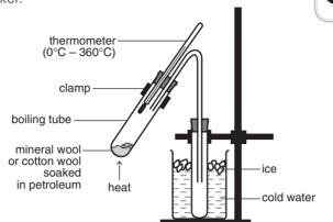
Heat the test tubes of contents gently. Collect the distillate in Test tube A. This is Fraction A.
